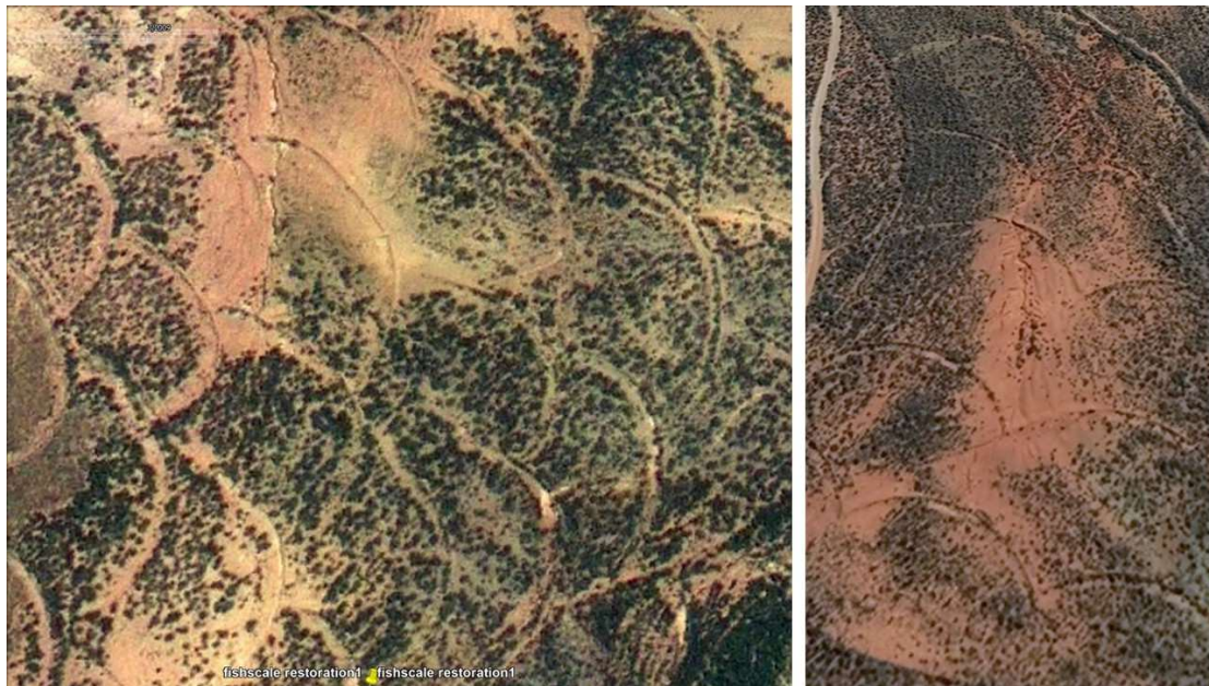
Figure 39. A large-scale fish-scale swale rehabilitation project near Montagu in need of maintenance. Accelerated runoff has broken through the swale dams and is causing on-going soil erosion.
